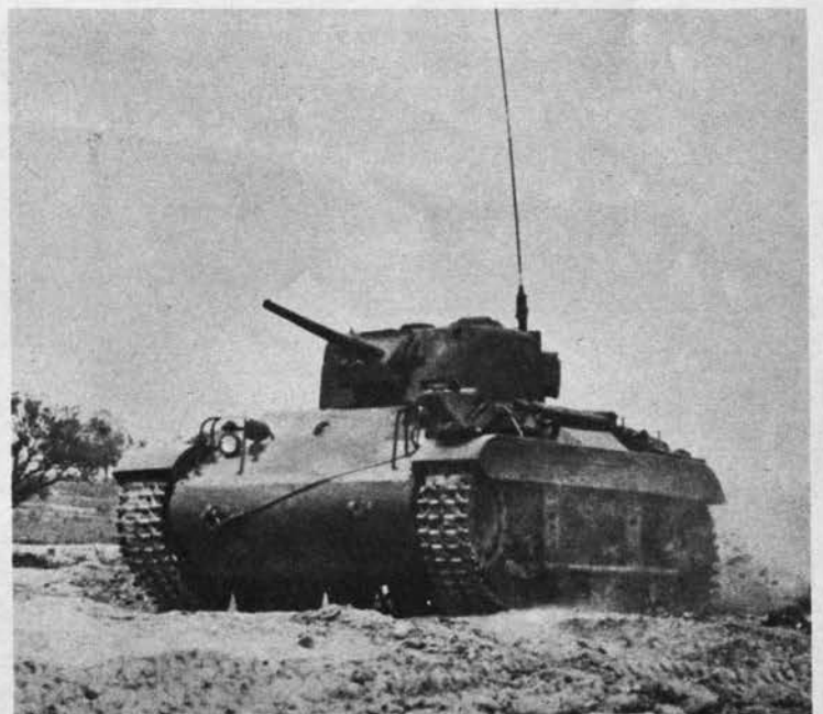
Vest-pocket M-22 is designed for airborne attack. It weighs eight tons, is 13 feet long and a little over seven feet wide. The hull lines are horizontal. Both the turret and the bow are smoothly rounded.
